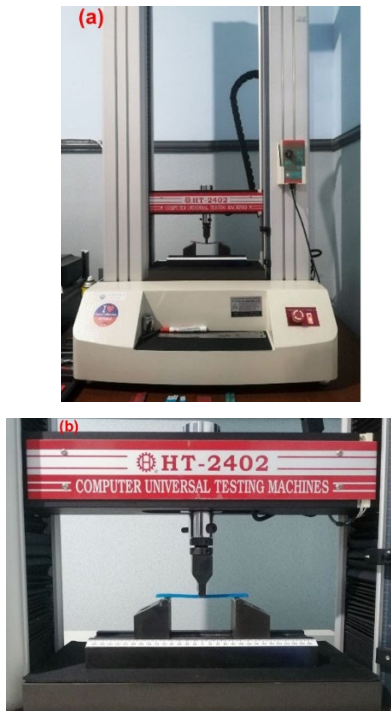
Fig. 2. (a-b) Universal bending testing machine HT-2402.
