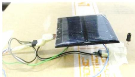
Figure 6. Position of light and temperature sensor placement at the time of testing
