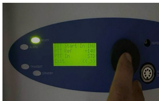
Figure 7. Display PTT Ref voltage -14 volts
