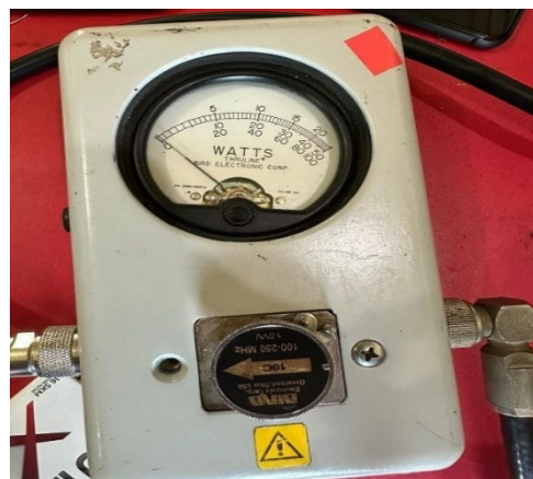
Figure 10. Measurement of reverse power value with element 10
