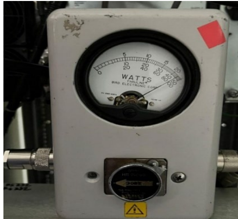
Figure 9. Forward power value measurement with element 250
